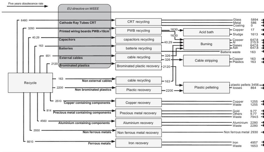
Fig. 3. Material flow of the post recycling processes of the tracer item personal computer within the system border Delhi in kilograms/day. Balance calculated for the year 2003.
