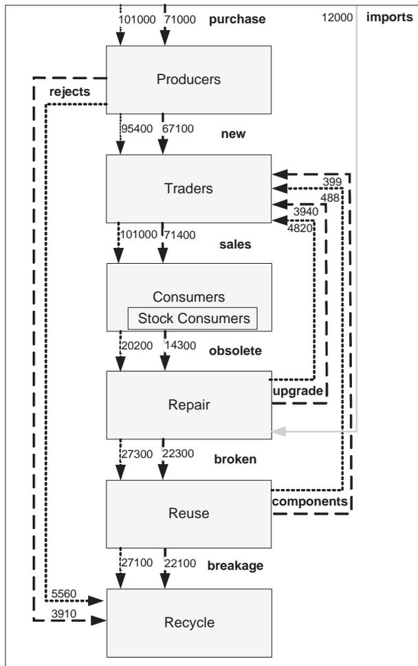
Fig. 2. Material flow of the pre-recycling processes of the tracer item personal computer within the system border Delhi in kilogram/day. Balance calculated for the year 2003. The stock of the process consumer is according to Table 3: 2,350,000 PCs (or 86,330,000 kg) plus “sales” minus “obsolete”, (rounded off at three and four digits).
