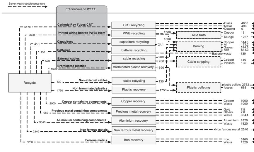
Fig. 4. Material flow of the post recycling processes of the tracer item personal computer within the system border Delhi in kilograms/day. Balance calculated for the year 2003.
